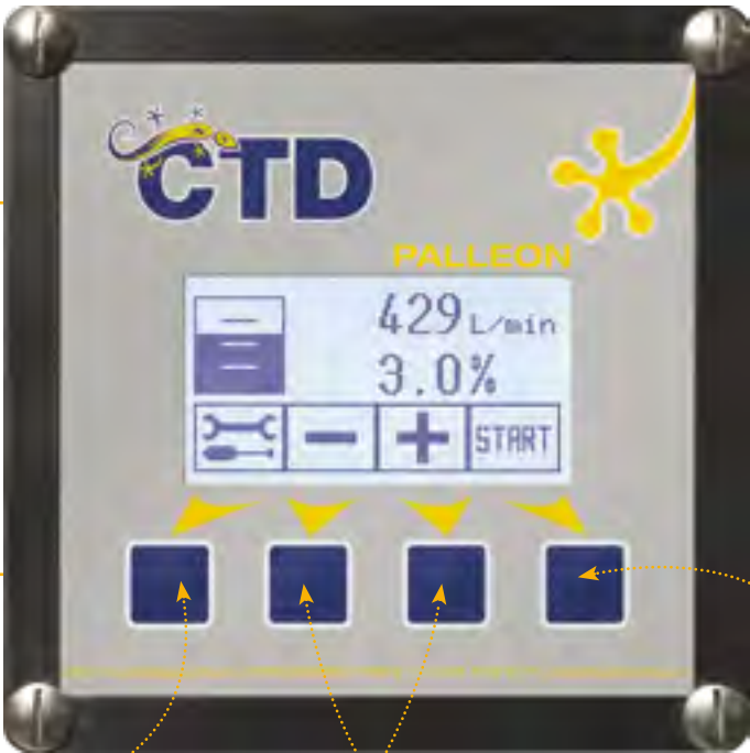
Configuration button Quick and easy selection of the desired CLASS B foam concentration (1 to 6 % in 0.1 % increments) Power START/STOP
